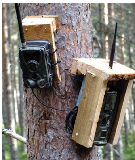
Cameras mounted on a Scots pine. The 700G is in a partial enclosure for extra protection.
