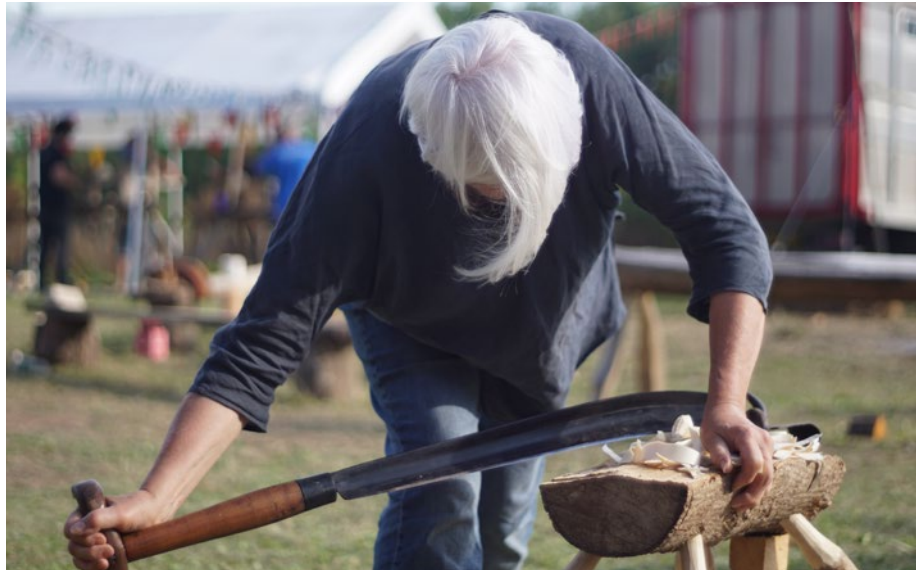
Using a paroir , an old French clogmaker's stock knife, to cut a blank.
