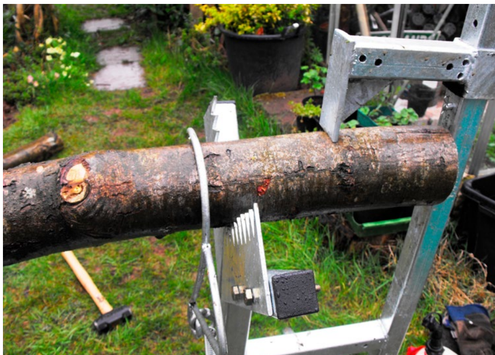
The log holder, with log firmly held in place in the teathed jaws and spring holder.
