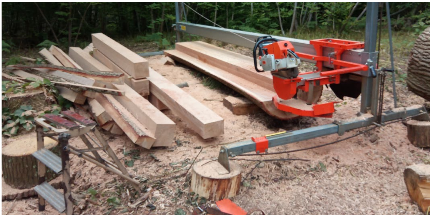
Above: swing arm mill, powered by a large chainsaw.
