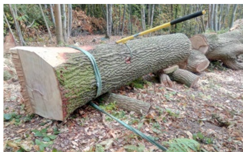
Above: rolling an oak butt off the stump and onto bearers with a hand winch ready for milling. The butt can also be skidded on to bearers by attaching the strop to the bottom of the log. This means you can get it into the most efficient orientation for milling. Take extreme care and carefully plan each move using chocks and wedges.
