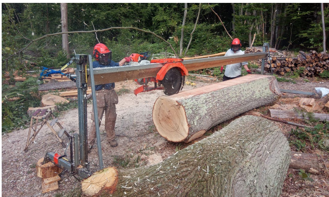
Setting up a swing arm chainsaw mill.
