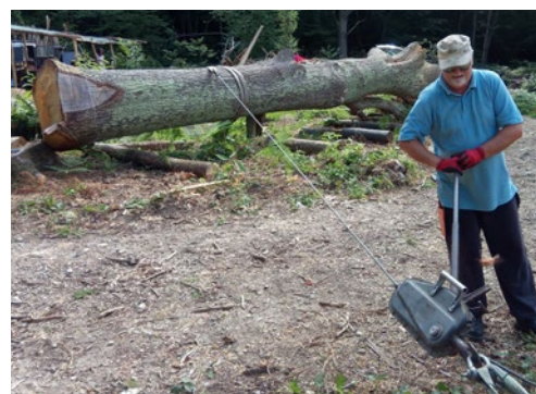
Above: swing arm mill, powered by a large chainsaw.
