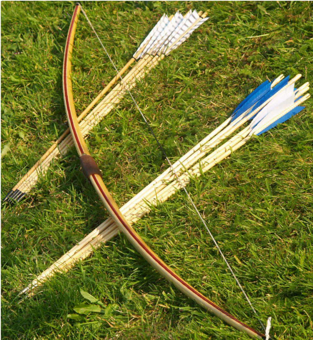
A trilaminate bow, made from a triple laminate of hickory, purple heart and lemon wood.
