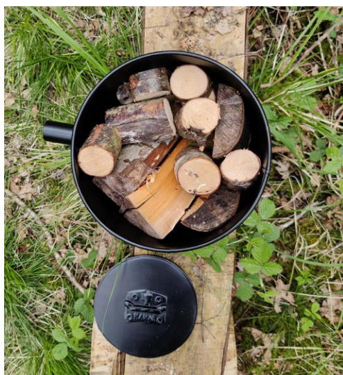
The smart black drum is packed with small logs and branches up to about 30 cm long. Make sure the drum is filled to the brim, then fit the lid.
