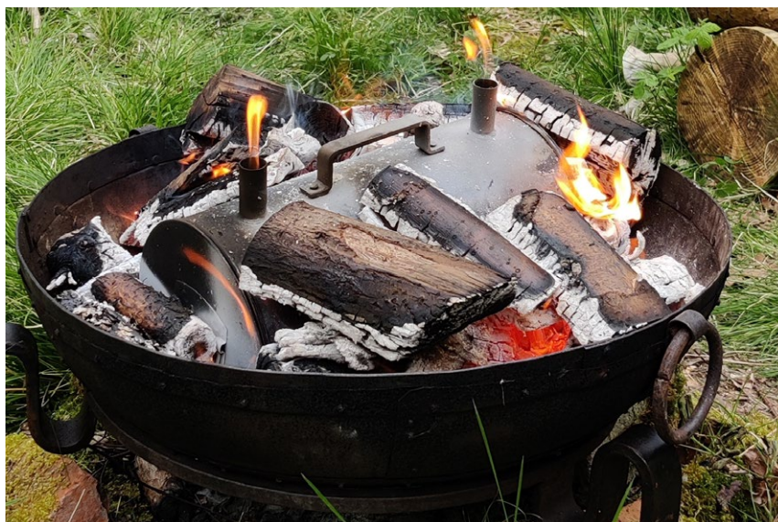
After about 90 minutes, flames appeared from the top vents and the doors of the drum, demonstrating that the wood gases were being burnt off as part of the process of pyrolysis.
